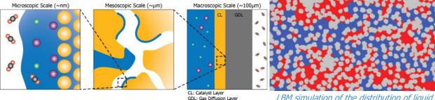
Different physical scales in Gas-Diffusion Electrodes used in CO<sub>2</sub> reduction. This projects supports **mesoscopic-scale** modeling by developing tools to **model dissolution of CO<sub>2</sub>** (white) in the **electrolyte** (blue).
