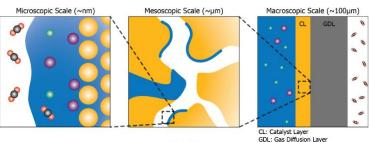
Different physical scales in Gas-Diffusion Electrodes used in CO<sub>2</sub> reduction. This projects supports **mesoscopic-scale** modeling by developing tools to **model wetting of the electrolyte (blue) and gas** (white) on the solid catalyst (yellow)
